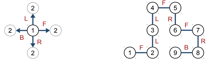
Figure 2: Internal coordinates representation based on absolute moves. Encoding scheme (left). Example conformation encoded as FLLFRFRB (right).
